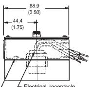
Electrical receptacle 8-32 Tapped hole for customer to connect ground
