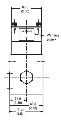
Electrical conduit connection is over solenoid on single solenoid models, and over "b" solenoid on dual solenoid models. See diagram plate for "b" solenoid location.
